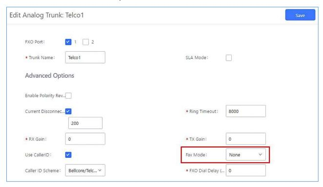
Figure 201: Configure Analog Trunk without Fax Detection
