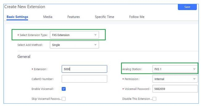
Figure 202: Configure Extension for Fax Machine: FXS Extension
