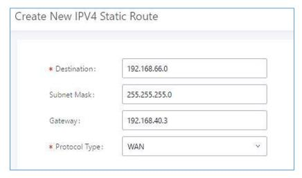
Figure 20: UCM6204 Static Route Configuration
