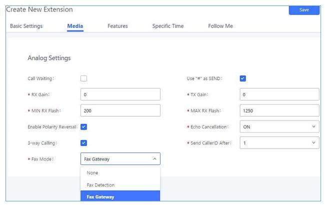
Figure 203: Configure Extension for Fax Machine: Analog Settings
