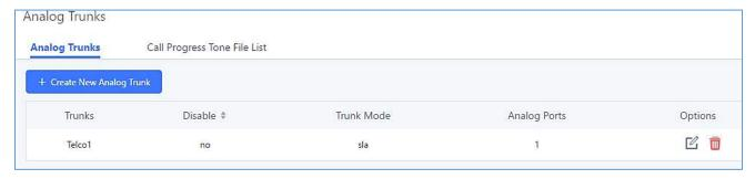
Figure 109: Analog Trunk with SLA Mode Enabled
