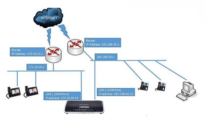
Figure 13: UCM6202 Network Interface Method: Dual
