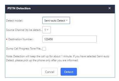
Figure 101: UCM6200 PSTN Detection: Semi-Auto Detect
