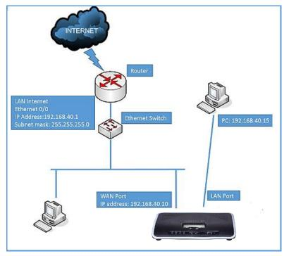
Figure 12: UCM6202 Network Interface Method: Switch
