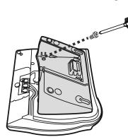
Mount the stand as shown and insert screw. Use the screw that came with your telephone.
