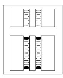
If you just want to cold start an individual module, on that module, simultaneously press the two top and two bottom buttons on the lower button set, as shown in the following diagram. The KIM displays a random pattern of icons as the KIM resets. • **KIM multi-module cold start** If you want to cold start all the KIMs attached to your telephone, simultaneously press the top two buttons on the upper button set, and the bottom two buttons on the lower button set, as shown in the following diagram.
