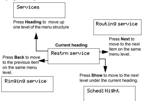
Programming buttons are active or inactive at different stages of programming. A button is active (meaning you can use that option), when the indicator next to it is lit ( $\blacktriangleleft$  or  $\blacktriangleright$ ).
